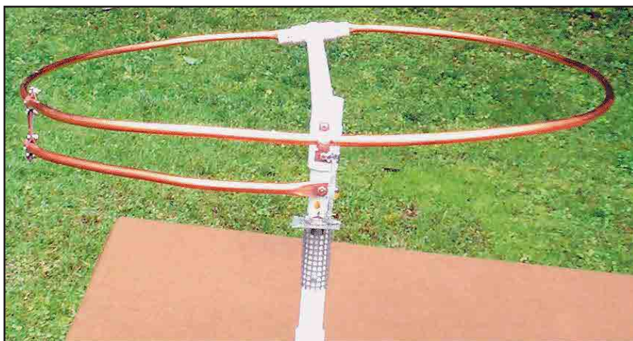
Figure 2—The halo from the rear. A copper strap connects the matching section to the halo on the left.
