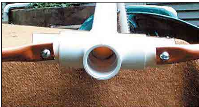
Figure 3—A block of wood and a hammer was the precision tool used to flatten the far ends of the halo.
