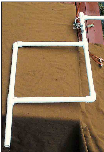
Figure 5—The loop mounting structure. A word of caution—plan how you will assemble the square carefully. With PVC adhesive, you don't get a second chance!
