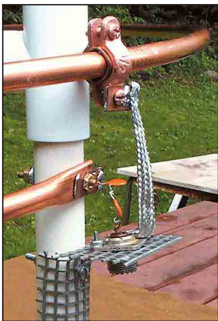
Figure 4—Details of the feed connection. The flattened tube approach could be used instead of the clamp shown on the loop on top.
